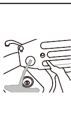
Drain the water out of water tank
